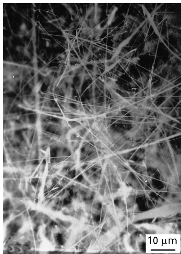
Figure 1 Scanning electron micrograph of wool-like AlN whiskers.
