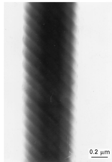
Figure 5 Transmission electron micrograph of a whisker grown by the axial screw dislocation mechanism.
