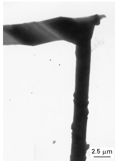
Figure 6 Transmission electron micrograph of a whisker with the axial screw dislocation turning to another direction.
